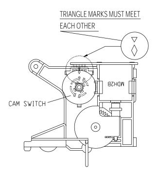
Fig.43 DATUM POSITION OF CAM SWITCH TRIANGULAR MARKS
